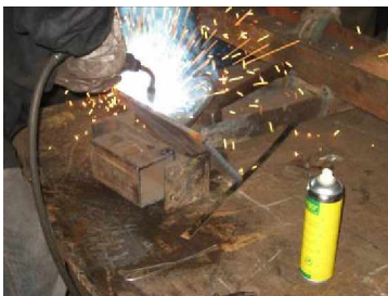
Fusing the Spray-can with „Bag-on-Valve“-technology is not hazardous since only the compressed air discharges
