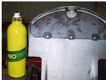
Refillable Spray-can by PROTEC with compressed-air-valve at the bottom for the Anti-Spatter protection
